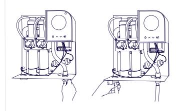
4. run faucets to purge air, secure wire leads to termial block, and ground
