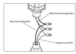
5. Make the following spliced wire connections using wire nuts:
