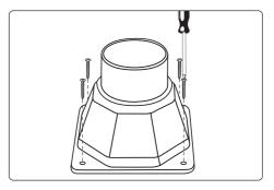
3. Screw the mounting base onto mounting surface, with base screws.
