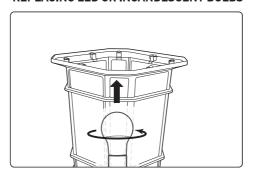
Unscrew to open top cover of post light, and remove the existing light bulb. Only replace light bulb with E26 base, 120 V, 60 W maximum.
