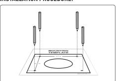
1. Select a mounting location suitable for supporting the light. Use the measuring template to mark the screw locations on the mounting surface.
