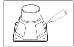
4. To prevent moisture from entering the mounting base, caulk the base to the mounting surface with silicone sealant (not included). The sealing compound should fully fill the gap of mounting base and mounting surface.
