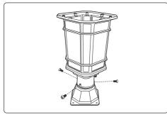
6. Carefully place all the wires and wire connections into the base. Attach the light to the mounting base, and ensure the orientation of the light is correct, with the light sensor facing front. Secure the light to the mounting base with set screws.
