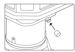
(Optional) To turn on the light during the day, place the Cap over the light sensor to disable the dusk-to-dawn feature.
