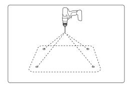
2. Wear safety glasses before drilling pilot holes. Drill four 1/16" diameter pilot holes.
