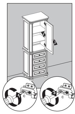
7. The cabinet is set up for the door (E) to open to the right side. To reverse the direction, unscrew the screws holding the hinges from the inside of the cabinet, and gently separate the door from the cabinet.
