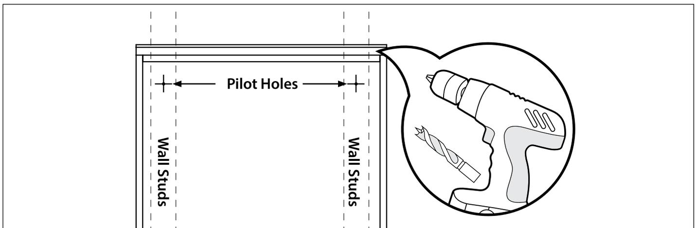
**4** Place cabinet flush against the wall and attach using screws and washers.
