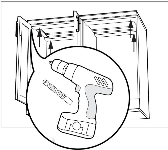
**11** Tighten screws to secure cabinets.
