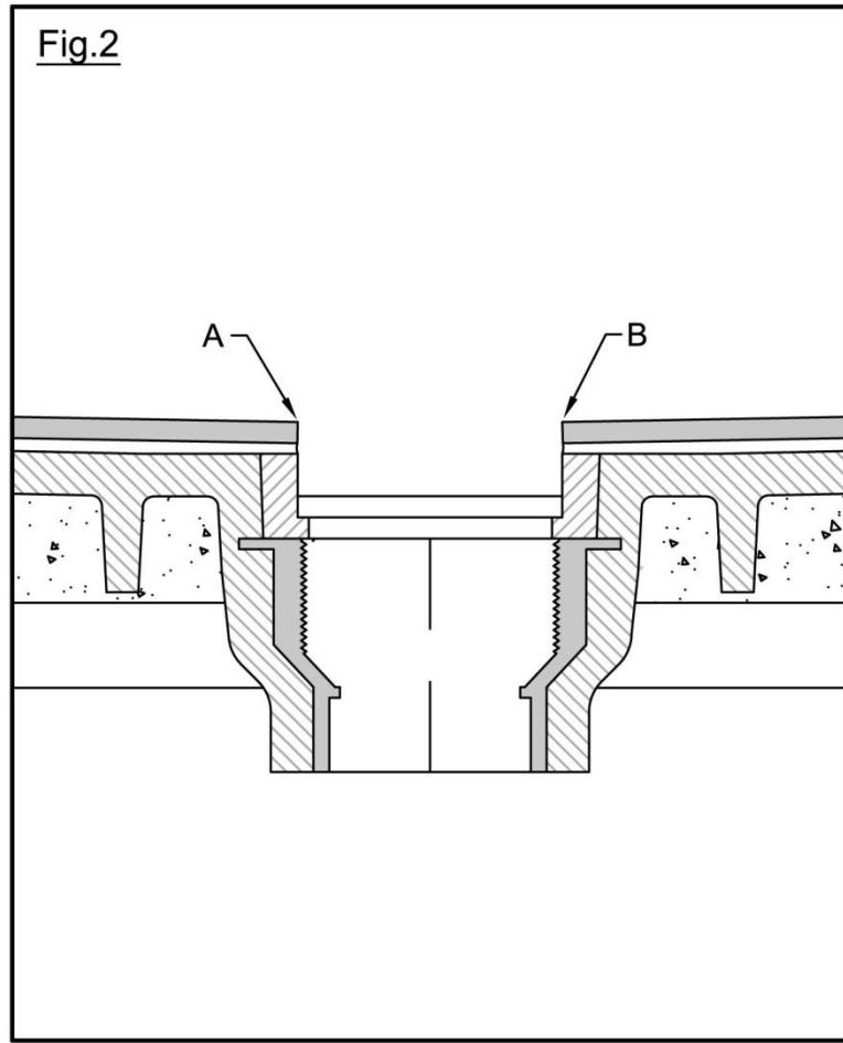
**III. HOW TO INSERT THE SOLID DRAIN GRATE INTO THE TILED SHOWER PAN SO THAT (A) IT IS SPACED CORRECTLY FOR DRAINAGE AND (B) IT IS AT THE SAME LEVEL AS THE ADJACENT TILE: (See Figs. 1 & 3)**
