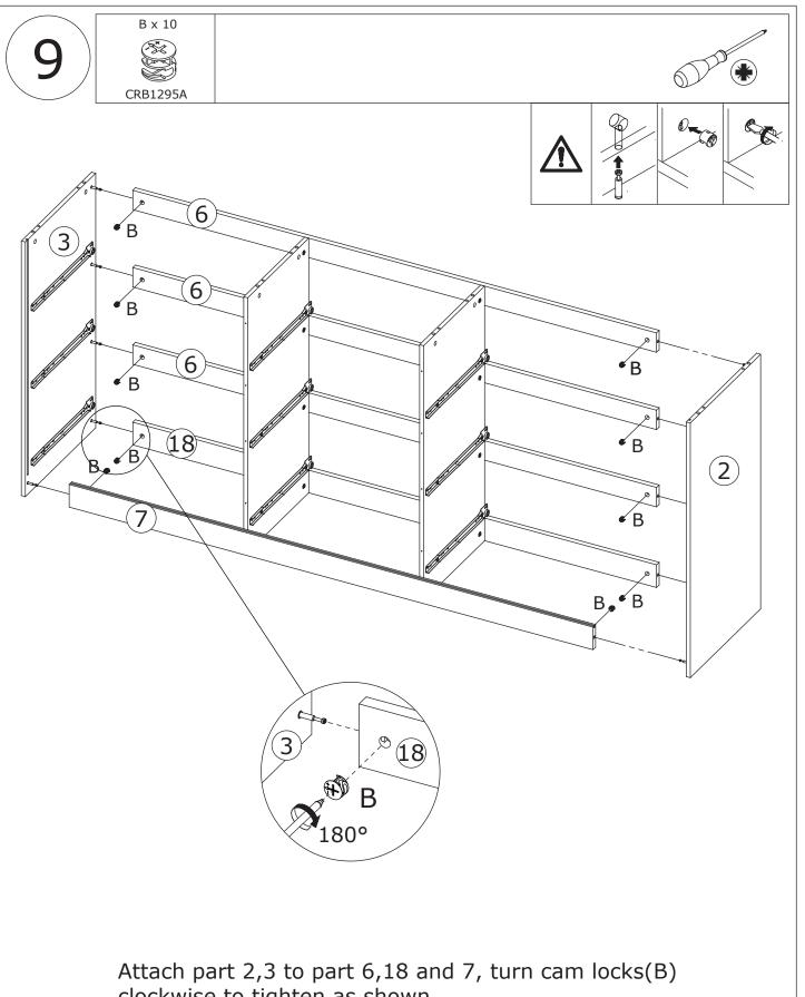
Attach part 2,3 to part 6,18 and 7, turn cam locks(B) clockwise to tighten as shown.
