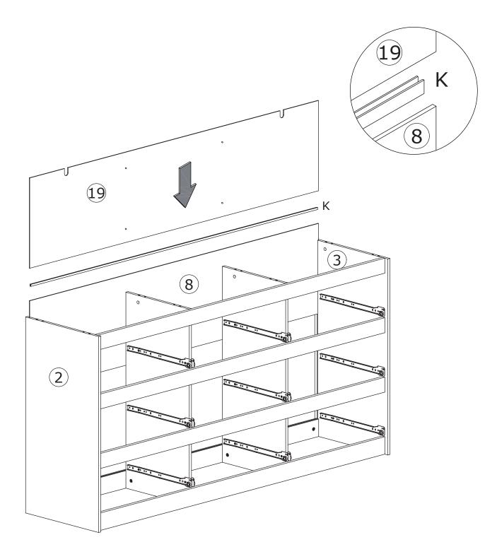
Connect part 19 and part 8 with part (K) and insert into the available slots of part 2, 3 and 7 as shown.
