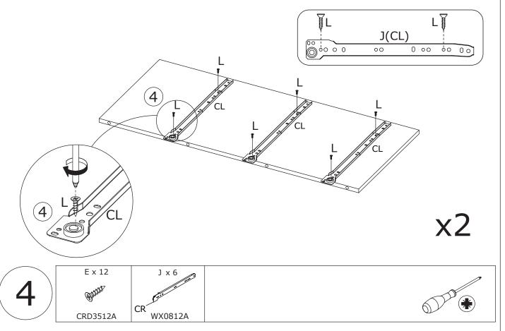
Fix slide rail(J) to the left of part 4 using screw(E) as shown. Please note, the pre-drilling of the rail on the right and left of this board is asymmetrical. Please install the rails according to the picture.
