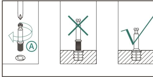
Tighten Ⓐ clockwise until all of their threads are engaged.
