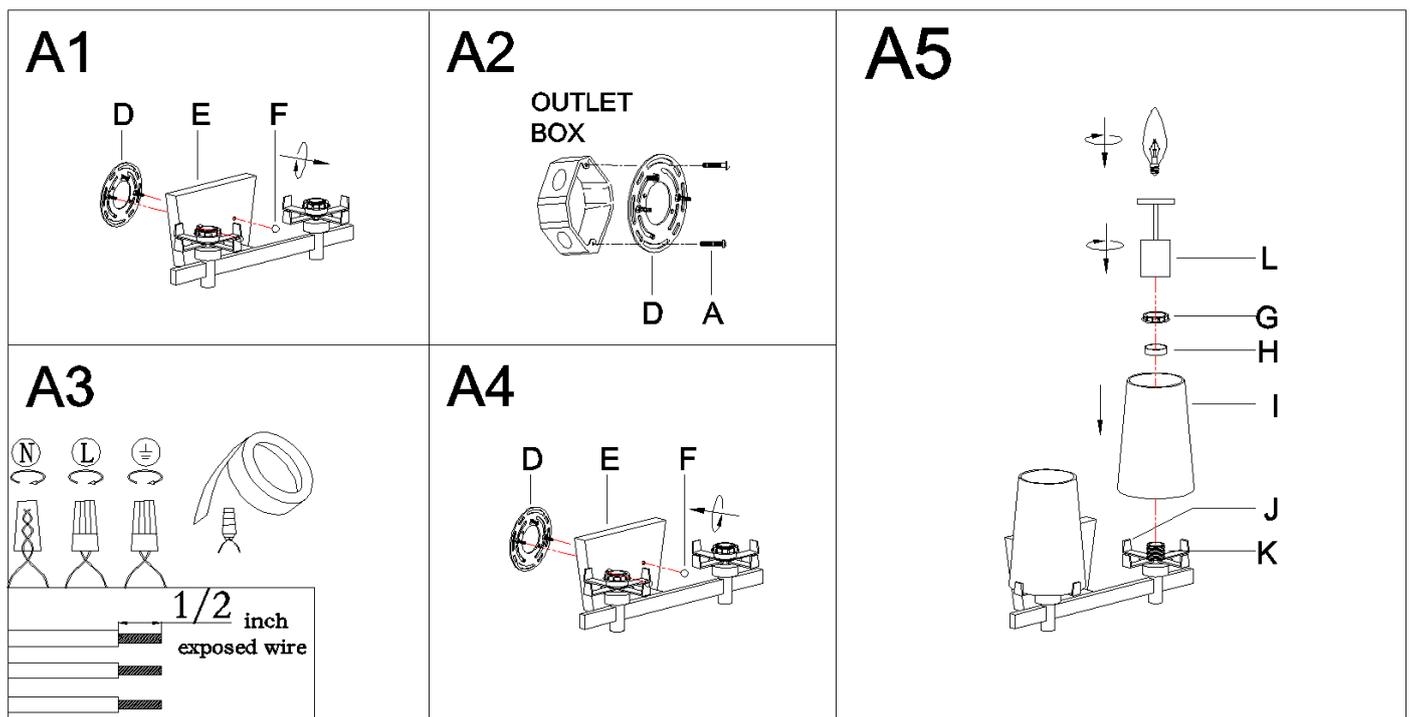
Step A1: Unscrew ball knobs (F) from back plate (E) then gently remove mounting plate (D).
