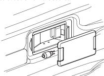
**NOTE:** To avoid damage or decreasing the life of the new bulb, do not touch bulb with bare finge s. Wear cotton gloves or use a tissue when replacing the light bulb.
