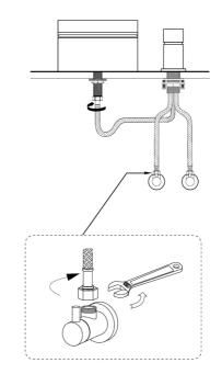
Connect the other side of red and blue water supply lines to the correct angle valves and use wrench to tighten them; Connect the other side of mixer water supply line to the spout and hand tight it(Don't use wrench in case of thread damage!)
