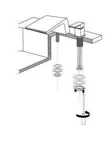
Screw plastic washers, metal washers and locking nut to the spout and handle part then hand tighten them; Use screwdriver to tighten the screws on Locking Nut B as picture2.
