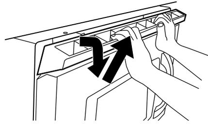
3. Slide filter back slightly, lift front end, and pull out filter.
