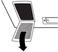
2. Replace grease filter by inserting one end of the filter into the back rim of the frame. Swing the front end of the filter up and slide it forward into position.
