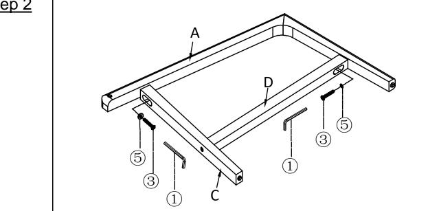
Attach the Front Left Leg (A) to Back Leg (C) and Support Left Leg (D), using Bolts (③), Washer (⑤) with Allen Wrench (⑥) as shown above.
