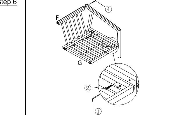
Attach the Back (F) and the Seat (G) to Right Frame, using Bolts (2), Screw (4) , with Allen Wrench (1) as shown above.
