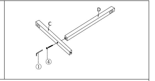
Open the carton and place all parts on a clean, non-marring surface. Attach the Back Leg (C) to Support Left Leg (D), using Screw (4) with Allen Wrench (1) as shown above.
