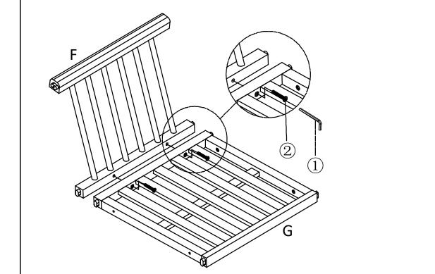
Attach the Back (F) to the Seat (G), using Bolts (2), with Allen Wrench (1) as shown above.
