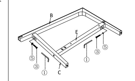
Attach the Front Right Leg (B) to Back Leg (C) and Support Rght Leg (E), using Bolts (3), Washer (5) with Allen Wrench (1) as shown above.
