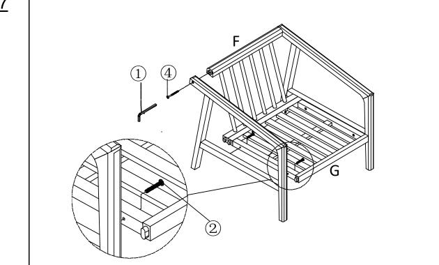
Attach the Back (F) and the Seat (G) to Left Frame, using Bolts (②), Screw (④), with Allen Wrench (①) as shown above.
