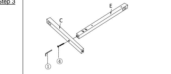
Attach the Back Leg (C) to Support Right Leg (E), using Screw (4) with Allen Wrench (1) as shown above.
