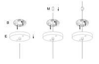
Note: Cuting the cord so that they are at least 6 inches (152.4mm) long within an outlet box and extend max. 3.1m long measured from the point where the cord emerges from the body of the lamp.
