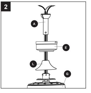
3. Slide the downrod (A) into the yoke of the motor assembly (G), align the holes, then re-install the downrod pin (B) and downrod clip (C). Secure with set screws (O).
