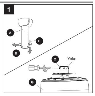
Insert the downrod (A) through the canopy (E) and yoke cover (L). Feed the wires from the motor assembly (G) through the downrod (A).
