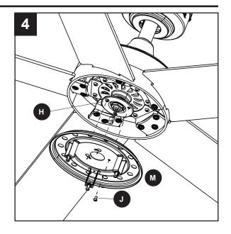
Remove one of the three light pan screws (Q) from the light pan (M) and loosen the other two screws. Connect the 9-pin connector from the motor assembly (G) to the light kit (I). Align the screw holes of the light kit (I) with the loosened light pan screws (Q) andturn clockwise. Replace previously removed light pan screw (Q). Tighten all screws.
