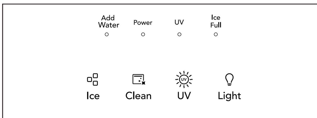
Plug in the power cord, the power indicator is on: you can operate this appliance by touch the button on panel as shown above, the main function includes: ice, clean, UV and light.
