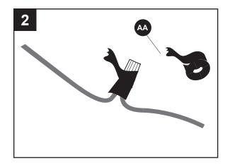
3. Turn the spliced/taped wires upward and gently push the wires and wire connectors (AA) into the outlet box.
