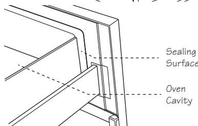
seals and sealing surfaces, broken or loose Microwave Drawer guides and dents inside the cavity or on the front side of the drawer. If there is any damage, do not operate the Microwave Drawer and contact your dealer or a SHARP AUTHORIZED SERVICER.
