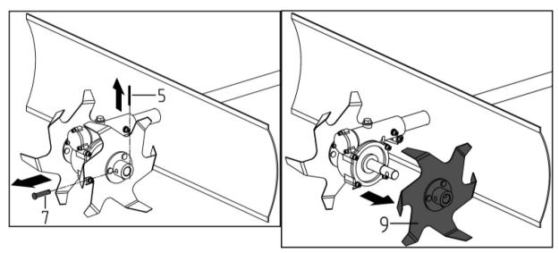
Install a new tines onto the cultivator/tiller according to the reverse steps of the above steps.
