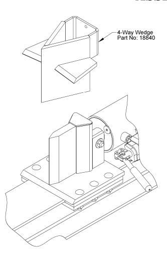
To install 4-way wedge, simply slide it over the top of the log splitter wedge ensuring it is fully seated. Ensure appendages are safe from any pinch points during installation.
