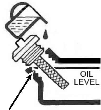
Figure 2 - Add Oil To TOP Of Threads
