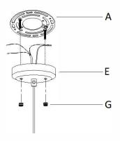
5. If needed, cut off the extra power cord length on the fixture 2 wires cord and green ground wire so that they all are at least 6 inches (152.4 mm) long within the outlet box
