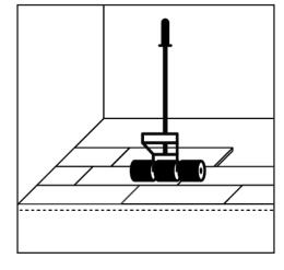
roller with extendable handle and your body weight or a 100 lb. three-section roller. Failure to roll correctly may result in bond failure. Repeat this process for the remainder of the installation. Remove all adhesive from the surface using a small amount of 70% Isopropyl alcohol and a clean cloth.
