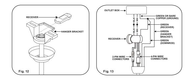
Step 1. Remove 1 of the 2 screws from the bottom of the hanger bracket and loosen the other one half a turn from the screw head.
