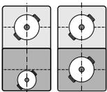
The front and rear elements with two inductors apiece can be used independently. The heat setting is set individually for each element. Use only one piece of cookware on each element.
