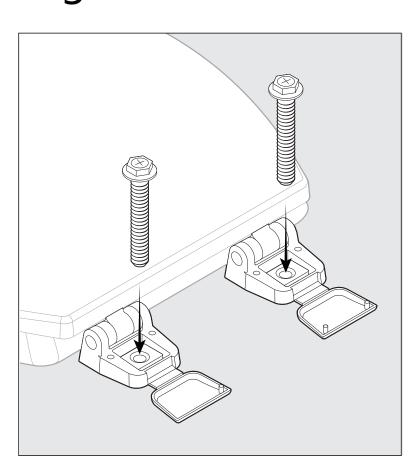
(4) Turn (B) onto (A) all the way up, finish finger-tightening from top
