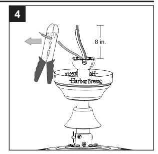
If you decided to cut back the lead wire in Step 4, strip 1/2 in. of insulation from the end of the white wire.
