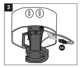
Align the canopy (E) over the loosened mounting bracket screws (G) preassembled on mounting bracket (D). Place the keyholes of the canopy (E) onto the mounting bracket screws (G) and rotate the canopy (E) clockwise.
