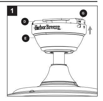
Secure the canopy (E) with the mounting bracket screws (G) previously removed (Step 4, page 8).
