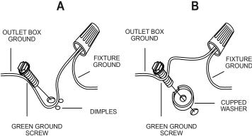
Connect wires according to the chart below
