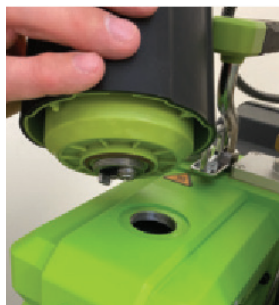
FIGURE 7: Demister removed, showing oil opening
