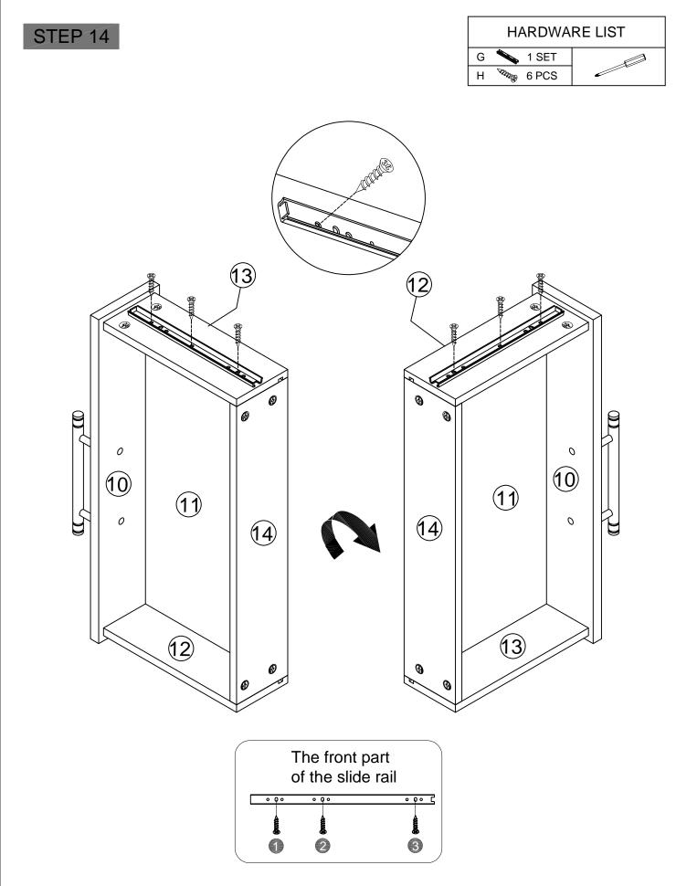
$^{\circ}$  The front part of the slide rail is attached to both side panels of the drawer using screws in the pre-drilled positioning holes
