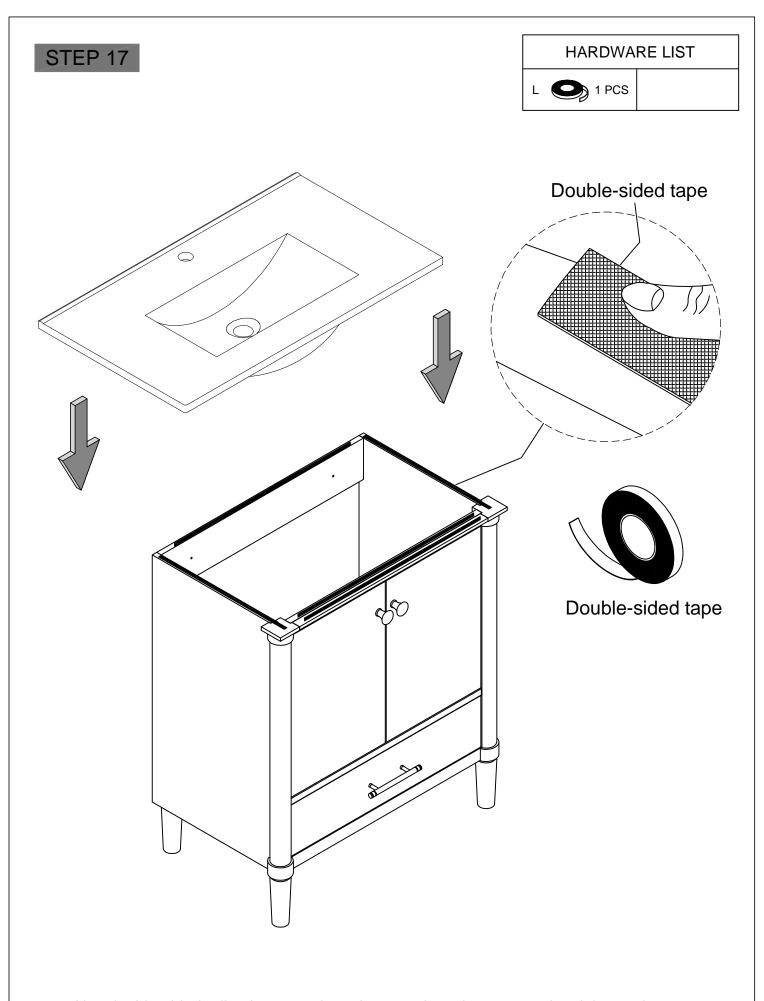
Use double-sided adhesive tape along the top edges that contact the sink to reduce wobbling when placing the sink on the cabinet.
