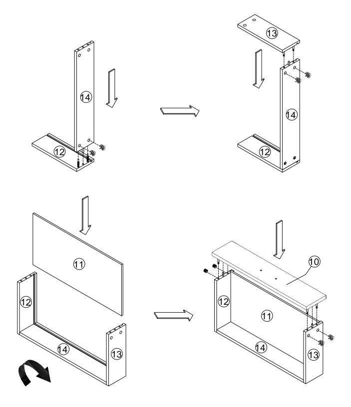
The side panels of drawer #12 and #13 are connected to the back panel of drawer #14 using Camlock, then the bottom panel of drawer #11 is inserted into the groove.
