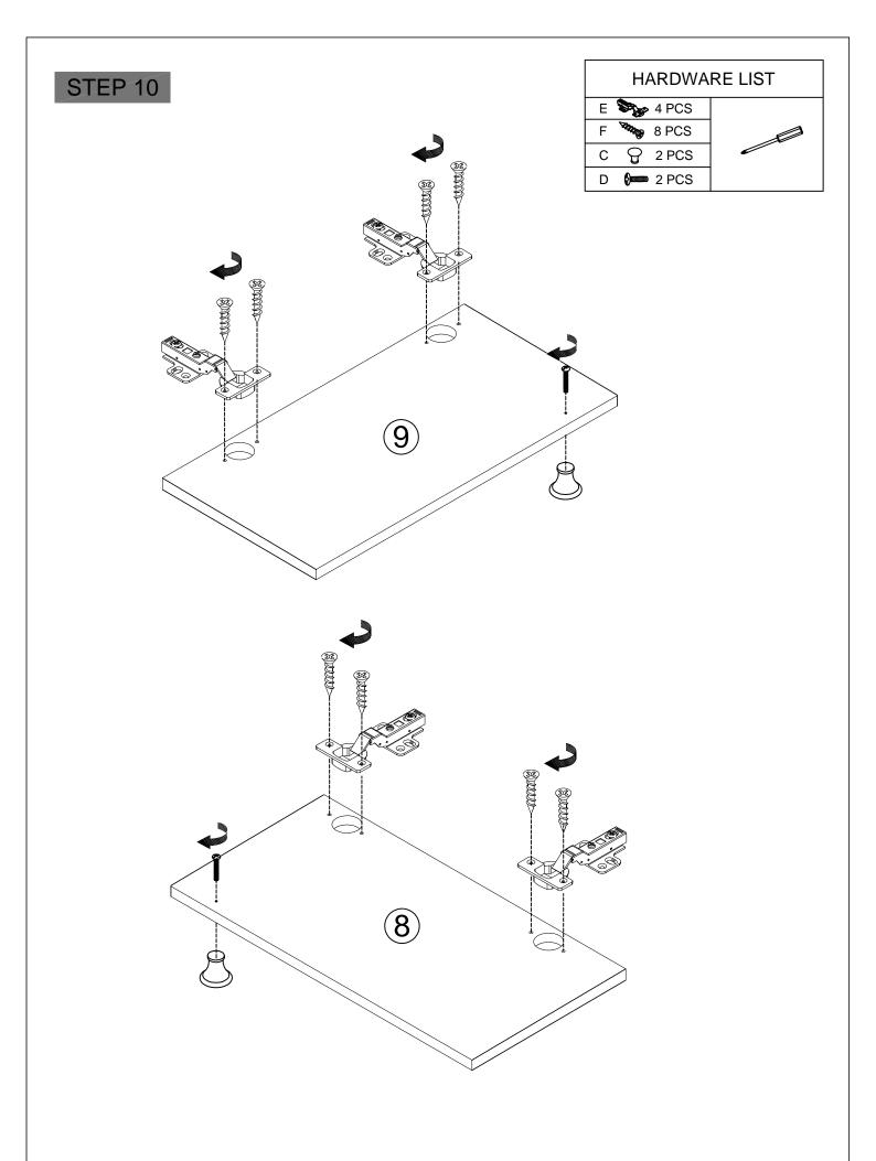
$^{\circ}\,\text{Use}$  Screws to install the handle and apply Screws to fix the hinge on the door #8 and #9
