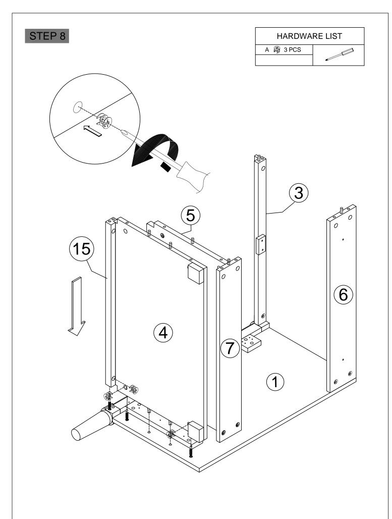
$\circ\,$  Refer to the illustration, already assembled #4 on the side panel. #1. Then tighten the cam lock
