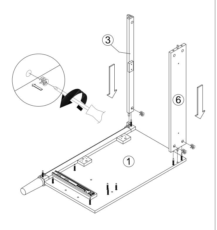
Refer to the illustration, already assembled #3, #6 on the side panel. #1. Then tighten the cam lock
