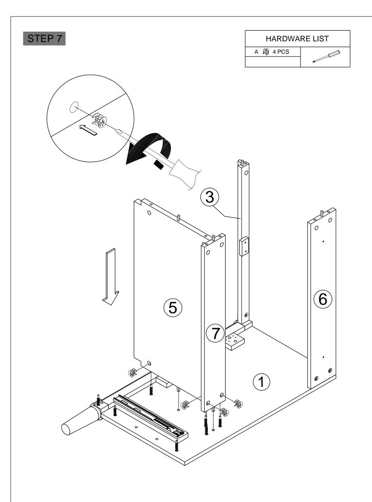
Refer to the illustration, already assembled #5, #7 on the side panel. #1. Then tighten the cam lock
