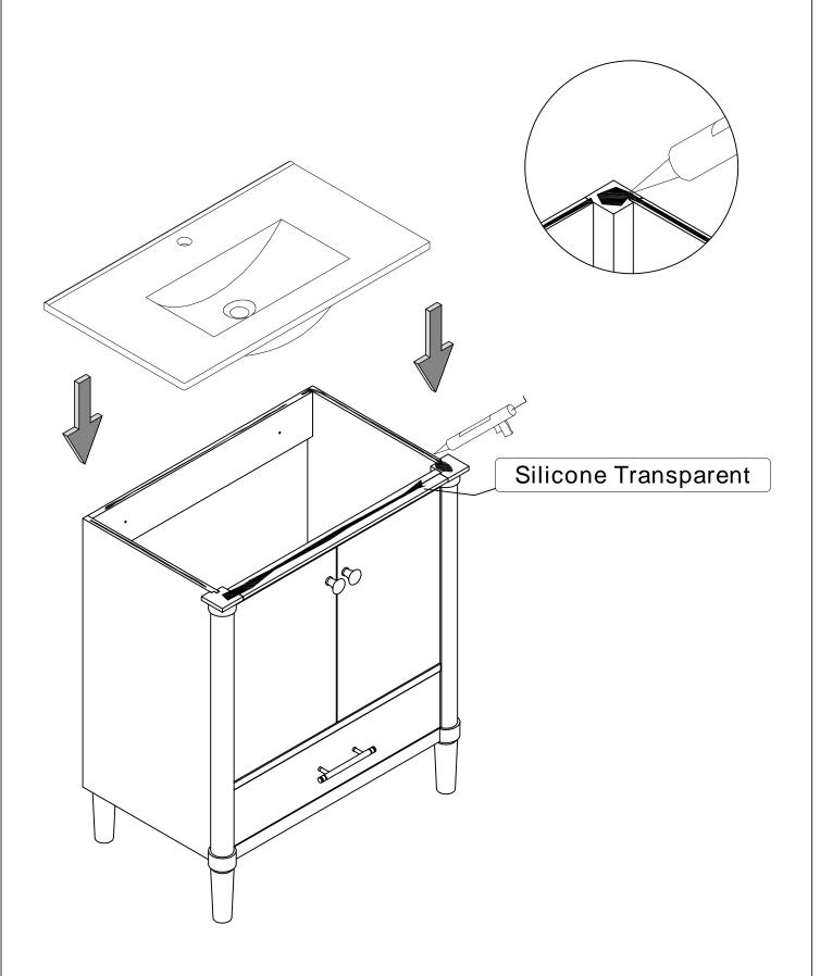
Alternatively, silicone adhesive can be used to secure the sink in place after positioning it on the cabinet.
