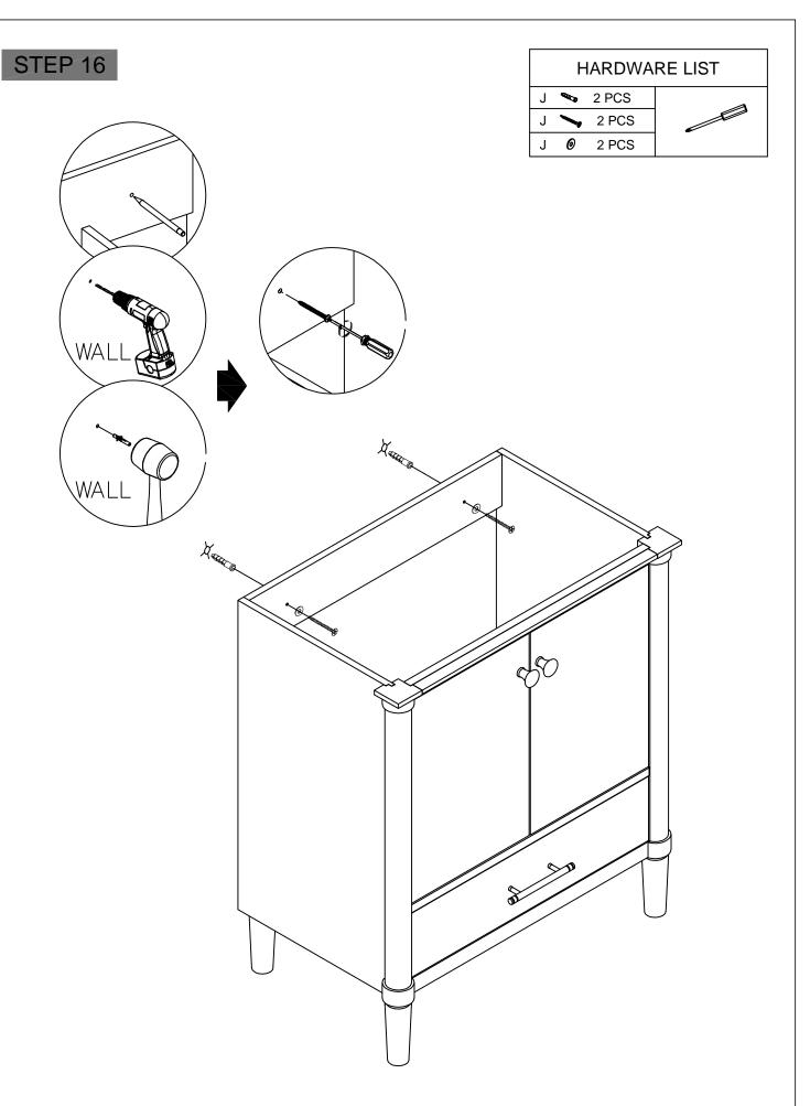
° Refer to the illustration, Draw the spacing between the walls on the cabinet, punch holes in the wall and fix the cabinet to the wall with screws.
