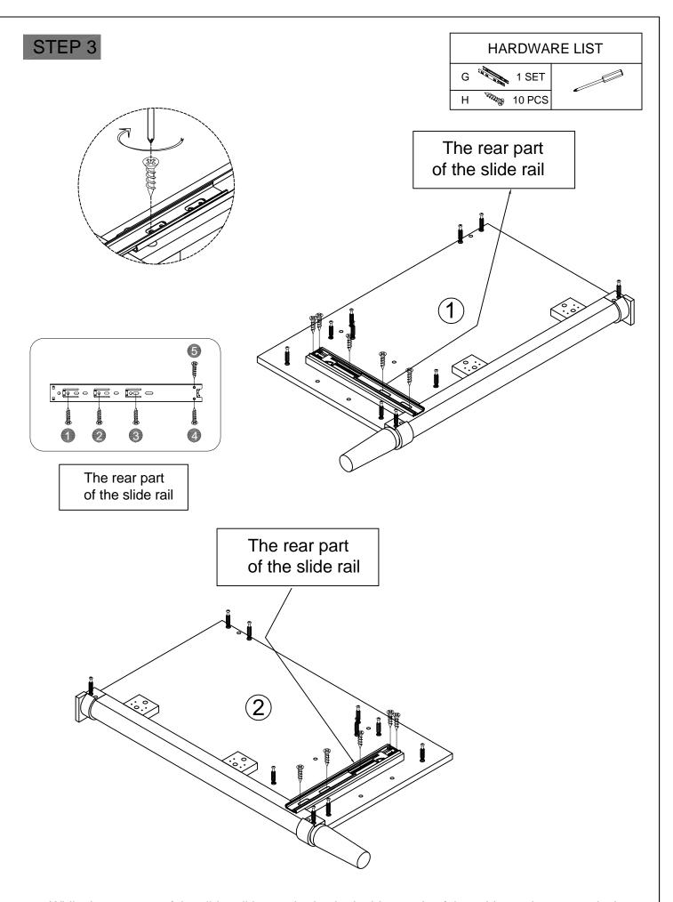
While the rear part of the slide rail is attached to both side panels of the cabinet using screws in the pre-drilled positioning holes
