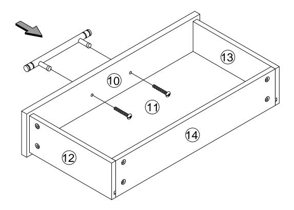
$\circ$  The front panel of drawer #10 is connected to the side panels of drawers #12 using Camlock , Use Screws to install the handle.
