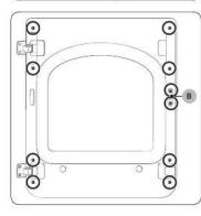
Locate and remove the 10 screws as shown. Note that screw B (x2) is longer than the others.
