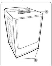
Using a level (A), check if the dryer is level side to side and then front to back. If the dryer is not level, adjust the leveling feet (B) at the bottom of the dryer. Then, check if the dryer is level again.
