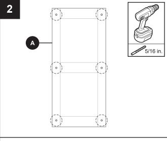
Drill a 5/16 in. diameter hole at each of the marks.
