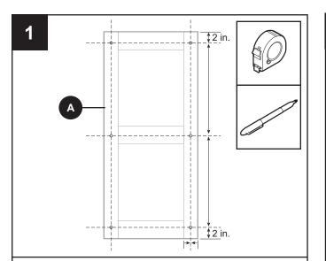
Lay the shutter (A) face up on a flat clean surface. Measure 2 in. down from the top of the shutter (A) and 2 in. up from the bottom of the shutter (A) and mark at the center of the side rail. Also mark at the center of side rail.
