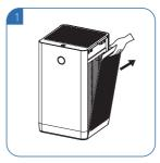
① Clasp the grooves of the left and right side panels by hand and pull diagonally upward and outward.
