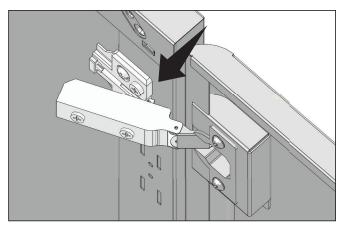
Align the hinge with the hinge plate.
