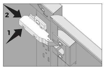
1. Press the back part of the hinge to click into position.
