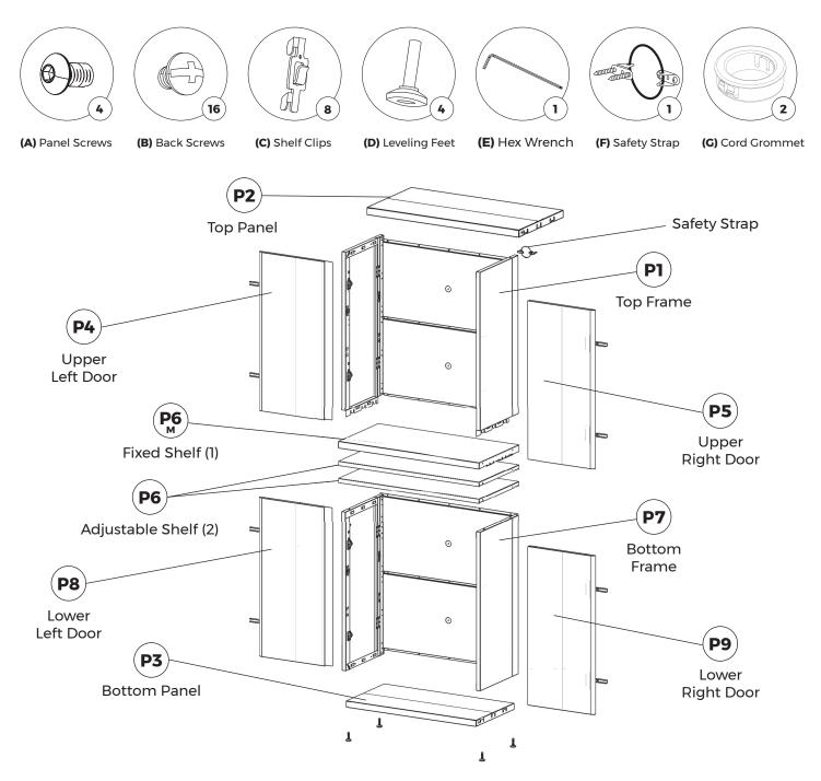
Remove both top and bottom frames **(P1, P7)** and lay on their backs on a protected surface with the sides facing up. Lift each side panel to an upright position.
