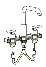
4. Push the blue button on the quick connect hose and insert the hose to the faucet and the handles' pipe as photo 4
