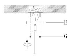
9. Install bulb (Not included) (Please do not exceed the maximum wattage recommended on the socket.)
