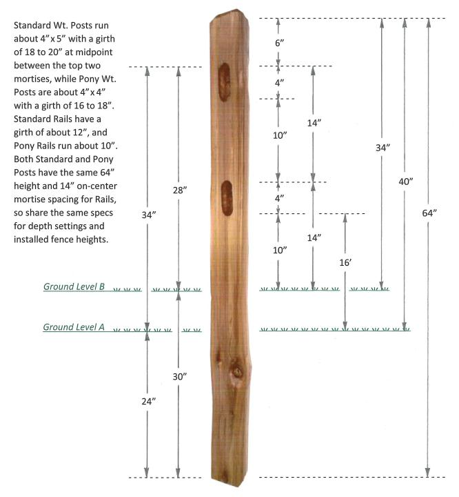
For **2-Rail Posts**, recommended depth is 24" (*Ground Level A*). Set at this depth, the tops of the Posts will be 40" above ground and the top Rails will sit about 34" high. This depth setting will leave about 16" clearance below the lower Rail.
