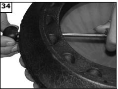
This step is for glass replacement only. Remove 1 glass holder and place glass in decorative body of light kit. Replace glass holder to hold glass in place.
