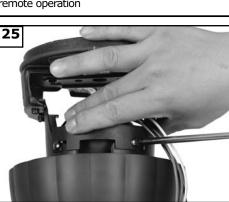
Re-install safety bar removed in step. 3 by placing safety bar on screws, sliding into place, and tightening the 2 screws.
