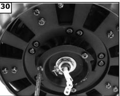
Loosen 2 of the 3 screws that will hold the light kit. Remove the screw that is associated to the closed hole on the light kit.
