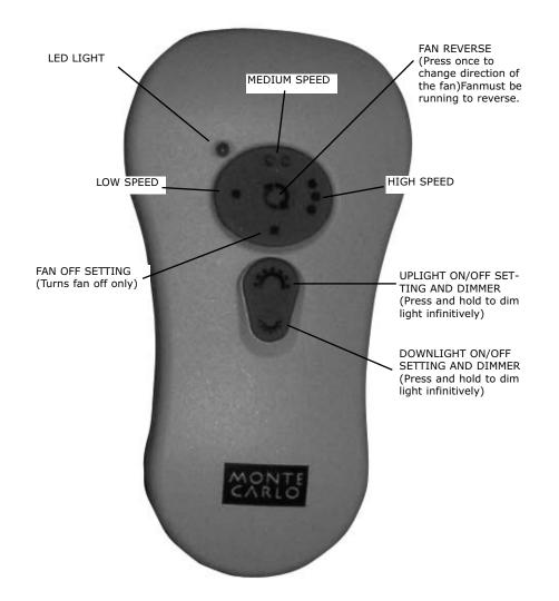
**FAN SPEED** Depress "I dot" for low speed, "2 dots" for medium or "3 dots" for high. To turn fan off press square".
