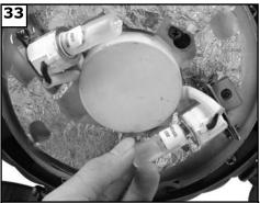
Install the 2x50 watt halogen bulbs. Do not touch bulb surface as oily residue from skin can cause the bulb to explode.
