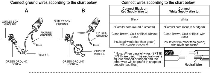
Twist wires together with plastic wire connectors (B) until tightly joined, and wrap each connector with approved electrical tape. Be sure that no wire strands are exposed and then carefully tuck all wires into the outlet box.
