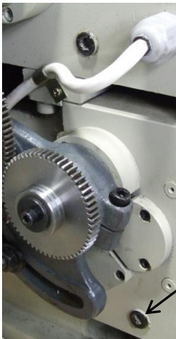
Gearbox Oil Drain
