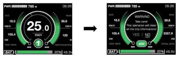
After clearance, the subtotal mileage TRIP is 0, average speed, and max speed is 0. Riding analysis is also 0. ODO information cannot be cleaned manually on the display, professional service tools are required.
