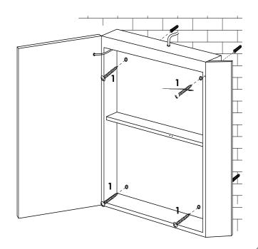
**Note:** When mounting to the wall, the wire can not be pressed between the cabinet and the wall, otherwise the wire installation will be affected.
