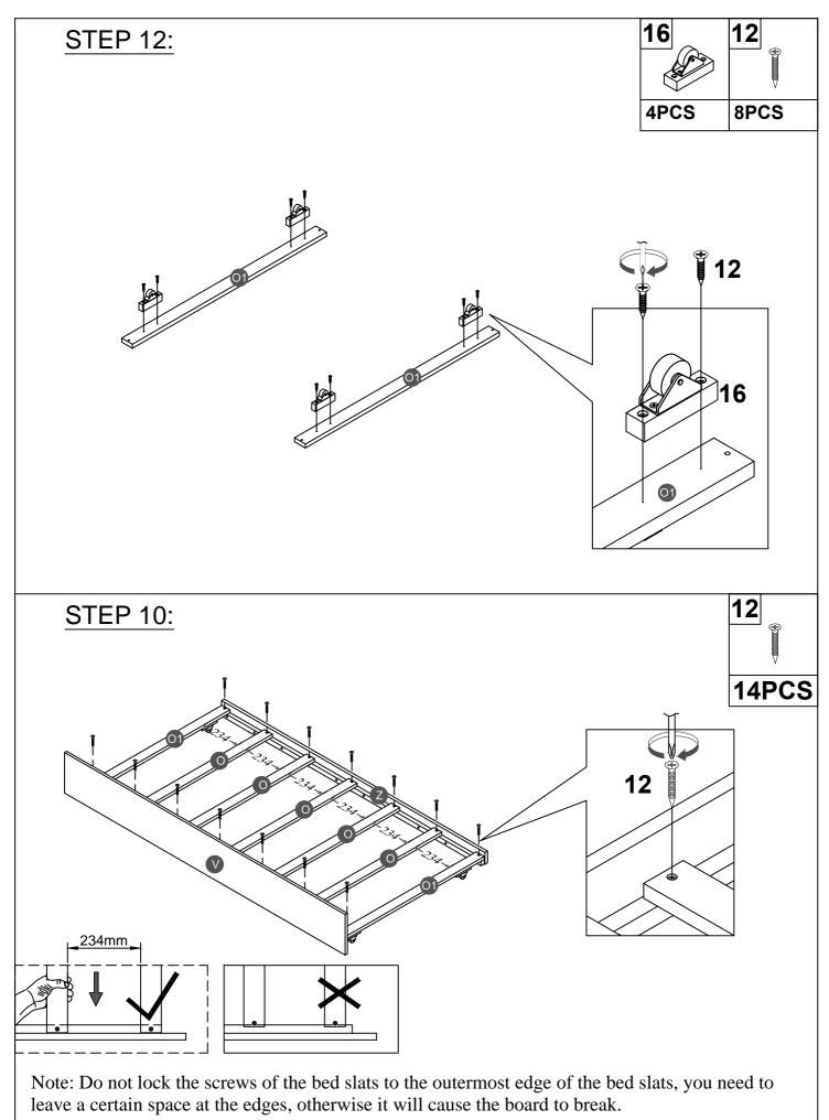
Do not lock the bed slats on the edge of the wood, please hold firmly before screwing, hold it in place with one hand, then lock the screw.
