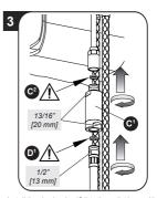
Install the check valve (C1) to the outlet hose with a rubber washer (C2) Secure with wrench Attach the pull-down hose to the bottom of the
