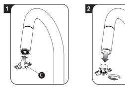
Before removing the aerator make sure that the faucet is turned off. Unscrew the aerator using the aerator installition key (E) included with the faucet if the aerator is clogged just rinse it with running water. Do not use detergents. Reassemble the aerator by following the instructions in reverse order.
