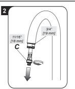
Disassemble the hose-carrier connection from the hand shower connection (C).
