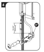
Attach the counterweight (D2) to the flexible hose approximately 15-3/4" [400mm] from the connection to the outlet pipe
