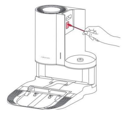
(6) Make sure that the front filter and the rear HEPA filter are not blocked. If there is any blockage, remove and clean it.
