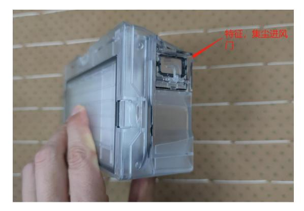
② Make sure that the plate covering the air vent is removed, as shown below.
