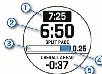
The device displays your target split pace ①, current split pace ②, completion progress for the split ③, distance
