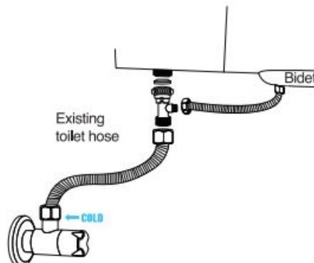
**Connect the T-valve under the toilet
