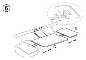
6. The Mouse Pad (D) attaches to the right or left side of the Keyboard Tray (C). Release the thumb screw on the attachment to move the Mouse Pad closer to or farther away from the Keyboard tray.
