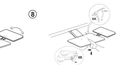
7. Press down to tilt the Mouse Pad and adjust its' angle. If the mouse pad is too loose, tighten the 2 screws on the mouse pad mounting bracket.
