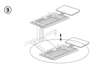
9. KT2 is adjustable from below your desk to above your desk. For fast adjusting: remove your mouse, release the lever (8A) & squeeze the handle (8B). When you've reached the perfect height, release the handle and then tighten the lever.
