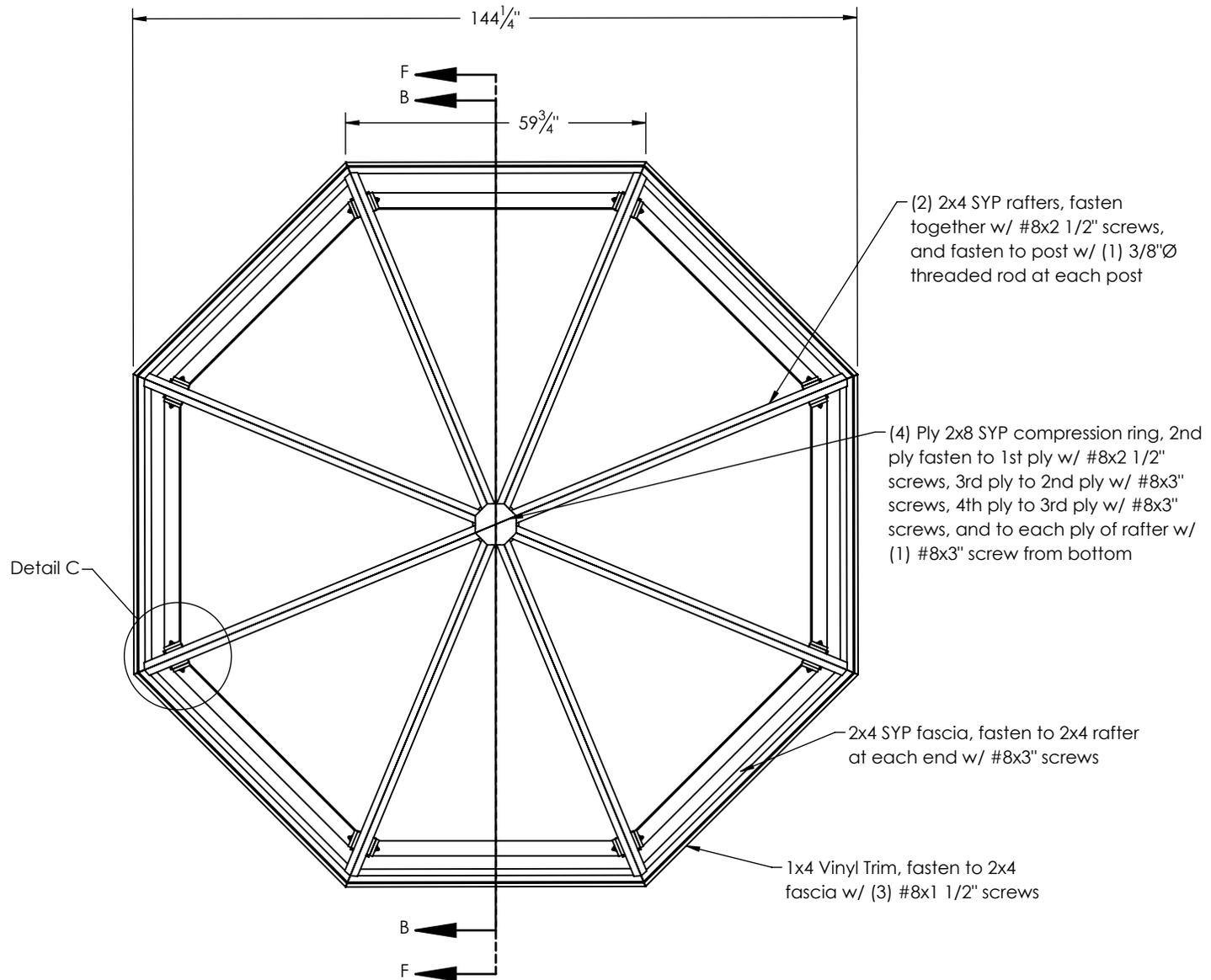
(2) 2x4 SYP rafters, fasten together w/ #8x2 1/2" screws, and fasten to post w/ (1) 3/8"Ø threaded rod at each post
