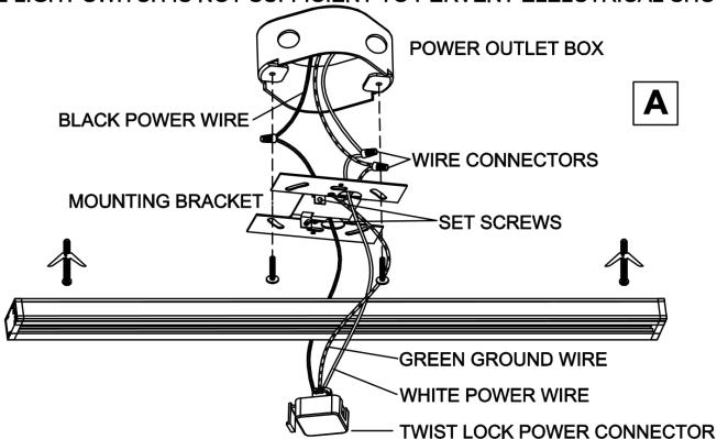
4. Check circuit load carefully, Themaximum electrical capacity of this track system is 15 amps per circuit for permanent installations. A standard 120V 15A circuit is designed to carry a maximum of 1800 watts, therefore, we recommend that the total wattage of all the lights and appliances persently attacked to the circuit should not exceed 1440 watts or 80% of the maximum electrical capacity.
