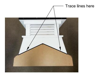
Cut along lines with a hand saw or jig saw.
